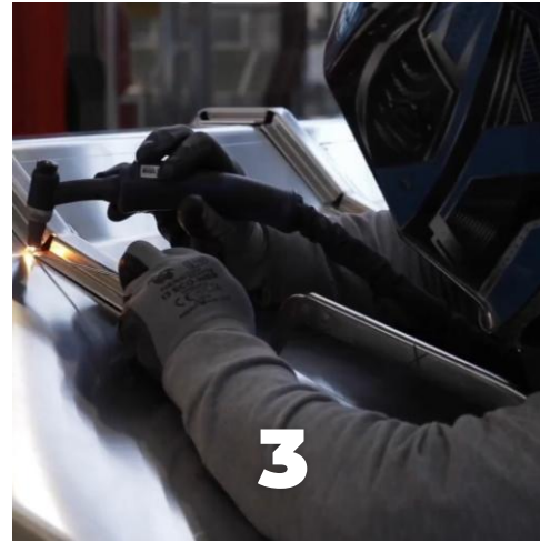
BODY IN WHITE (Welding and Bonding)
